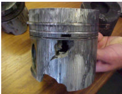
Figure 1: Hole through piston
