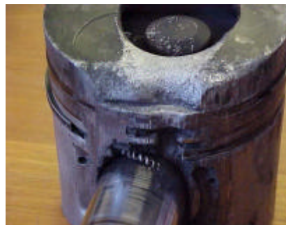
Figure 2: Melted piston crown
